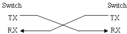
Figure 6-3 Fiber-Optic Cable Connection
